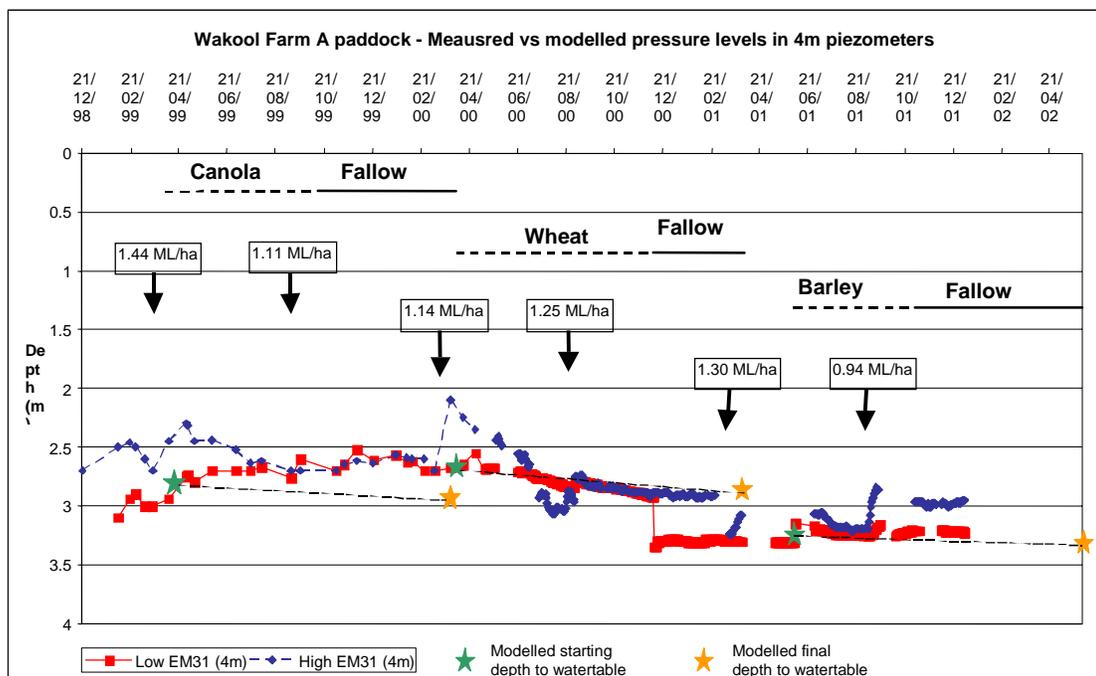
Figure 6 Validation of Lumped Model with Detailed Monitoring Data
