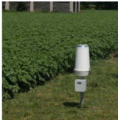
Photograph 2. Rain gauge mounted at IUNG agro weather stations (an example)
