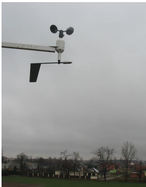
Photograph 3. Wind speed sensor mounted at one of IUNG's agro weather stations (an example)
