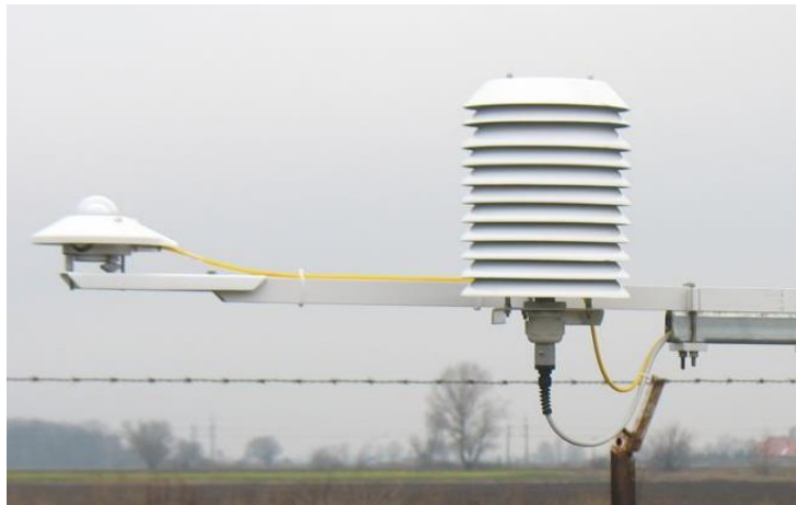
Photograph 1. Temperature and humidity sensor (Vaisala) mounted in a radiation shield (Aster – Polish manufacturer) and pyranometer sensor (Kipp&Zonen) mounted in one of IUNG's agro weather stations (an example).
